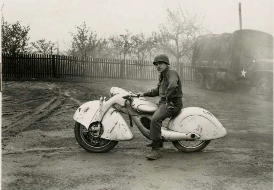
Photo No. 2 Left side. Note attachment of front fork to carburetor housing.
